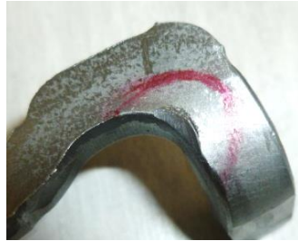
Fig. 6. Lane support (deformation)
