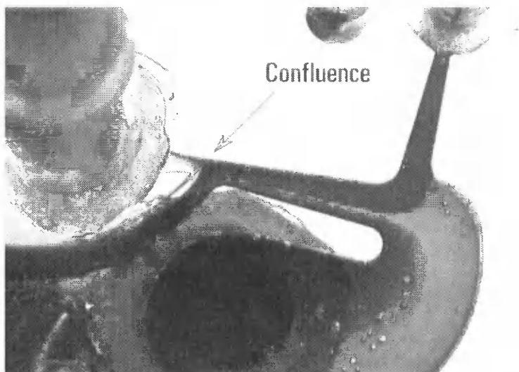
Fig. 4. Jet-pumping part of the valve in Phase A visualized by addition of a dark dye to the sample fluid flow. The small control flow just leaves through the output Y (Fig. 1) together with the sample fluid
