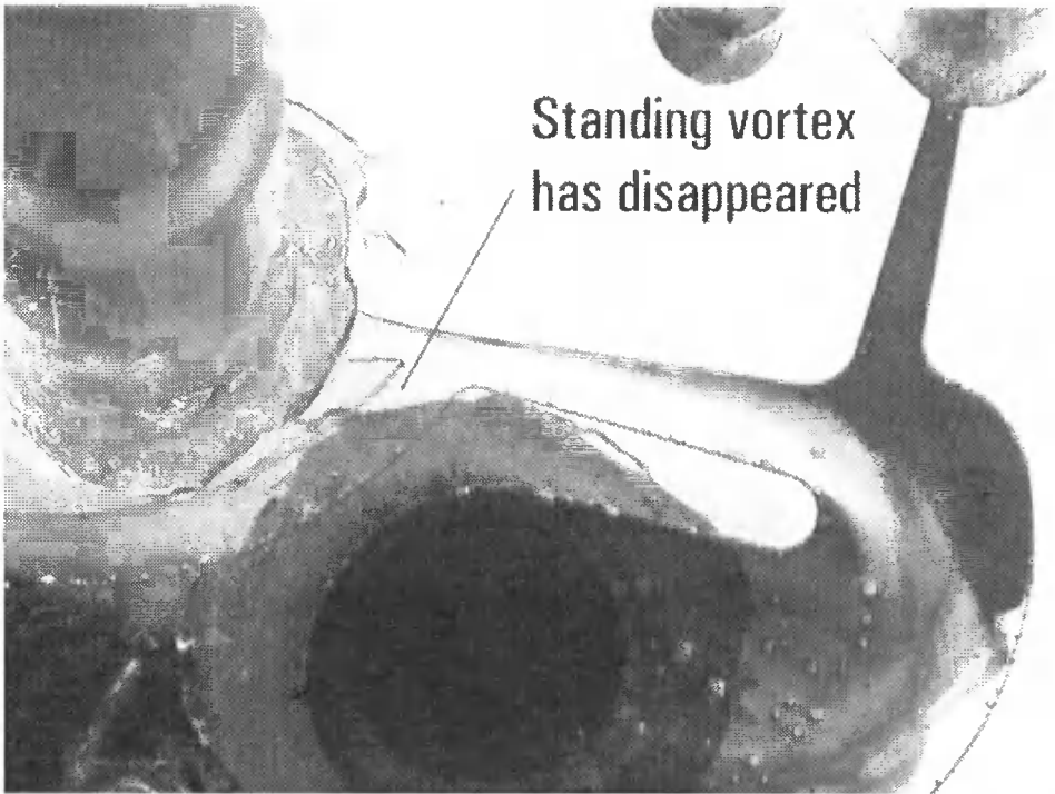
Fig. 7. Visualised fluid flow inside the valve in Phase B after some time has elapsed. The computation predicted large vortex was swept away with the flow into the output channel
