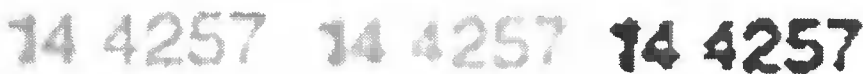
Fig. 3. Images of the digits: from the preprocessing stage, after filtration and after binarization
