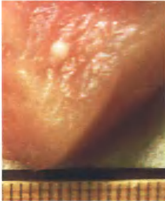
Fig. 8. Chicken breast interior exposed by axial cut after heating by microwaves using an antenna with h = 0.9 mm. Microwave pulse duration = 1.04 sec. f = 9.27 GHz. Extent of white region = 1.5 mm. Scale divisions are 1 mm in both Fig. 8 and Fig. 9.
