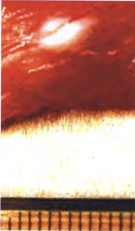
Fig. 9. Chicken breast interior exposed by axial cut after heating by microwaves using an antenna with h = 2.5 mm. Microwave pulse duration = 1.1 sec. f = 9.23 GHz. Extent of white region 5.5 mm long x 3.5 mm diameter.
