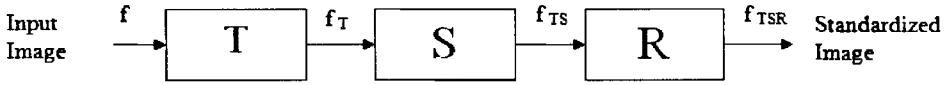
Fig. 3. Standardization of the input image which makes an object in processed images invariant to the translation (T block), scaling (S block) and rotation (R block)
